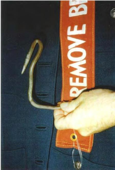
The pin in the picture at the left IS THE REAL ONE! The pin is suppose to be straight. Contact with a rotating propeller on a running Wright R-3350 engine created the multi angles shown. Somehow I managed to keep it with me all these years and it even survived a rather messy divorce in which I lost MUCH military memorabilia (including a couple of photo albums).
